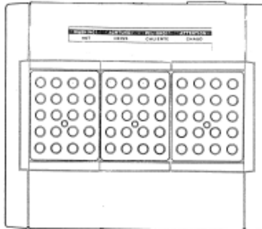
Top view showing three insert blocks in place
